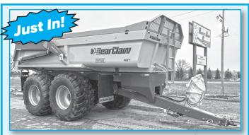
Bear Claw 40T Rock Trailer This beast has a load capacity of 40 ton. The hydraulic, up and over tailgate makes it a breeze for unloading.
